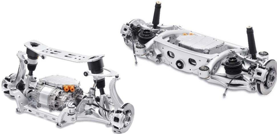
The integration of an electric powertrain in the chassis brings with it a significant increase in engineering complexity. BENTELER, with its Integrated E-Chassis Module (IEM), offers chassis system solutions for several vehicle platforms from B up to E segment for front and rear suspension. The key is scalability and modularity of the chassis.
